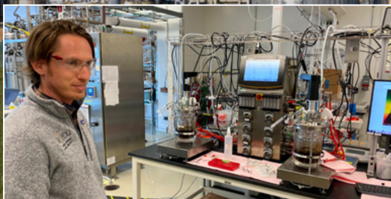
Lawrence Berkeley National Laboratory Research Scientist Eric Sundstrom with the lab-scale 2-liter reactor producing sugars from forest and agricultural wood.
